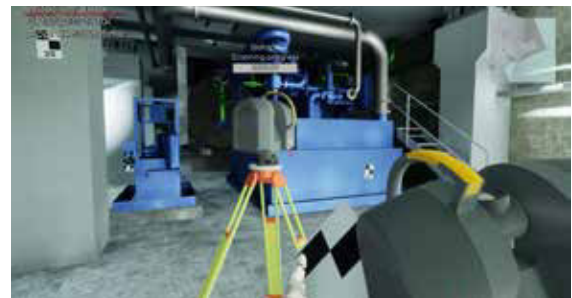
Target placing and laser scanner positioning in industrial environment in VRscan3D software
