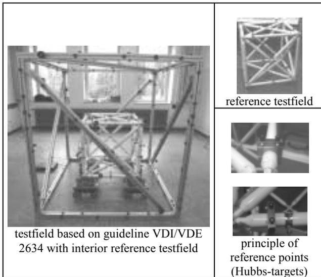
Figure 3: Testfields and reference points
