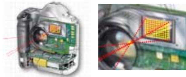
Figure 1: Principle of the correction grid applied for a digital camera (Kodak DCS)
